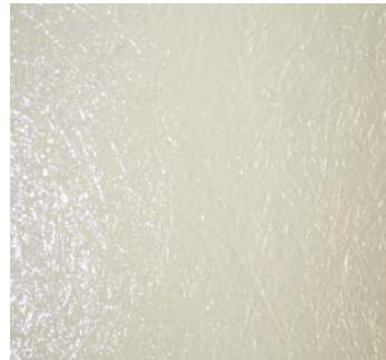
Surface 5 – Gel Coat Layer
