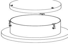
Water-resistant lids, "Type B" systems utilize pull downs latches to hold the lid securely against the sealing gasket on the reducer rim.
