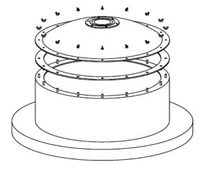
Water-proof lids, "Type A" systems are gasketed and secured in place with wing nuts, lock and flat washers.
