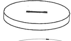
Friction fit, "TC" Lids simply slip over the reducer top.
