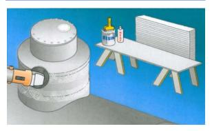
BE SURE TO WEAR A DUST MASK! Using a disc sander, with medium to heavy grit sand paper, scuff up all seam areas a minimum of 4" to each side of the point where the components will be bonded. It is very important that this be done fully, as the bonding materials will not adhere to any surface that has not been sanded. Brush sanding dust from seam areas.
