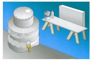
Apply additional coat of resin solution to seal sump surface.
