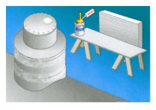
Add hardener, MEKP, to resin & putty. Hardener ratio at 70 degrees F. & 30% humidity is two (2) ounces per gallon for resin and one (1) ounce per gallon for putty. This will vary with temperature and direct sunlight. If used in direct sunlight or in temperatures above 80 degrees, reduce hardener as per instructions from supervisor or Western Fiberglass personnel. Mix thoroughly, scraping the sides of the buckets with the stir stick.
