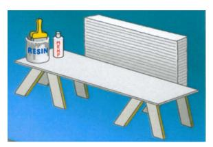
Using 1 layer of 3 oz FRP mat, lay out fiberglass mat for each seam to be bonded.
