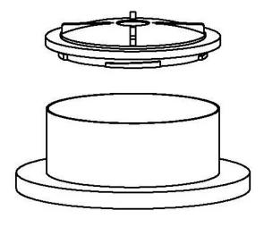
Water-proof "Twist-Seal" lids should be lubricated using white lithium grease. Align the arrows on lid with arrows on the side of the reducer. Turn clockwise until lid is firmly seated. Inflate gasket to 5-10 psi. To remove lid, deflate and unscrew.
