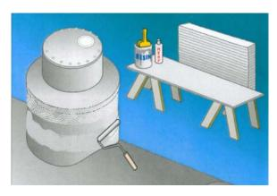
Use roller tool to "roll-out" air bubbles gently, so as not to displace putty. Remove all bubbles. Your laminate should appear clear, with no air bubbles or pockets in view and all fasteners covered.
